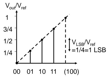
◆ A multiplying DAC (MDAC) is realized by simply allowing the reference signal, V<sub>ref</sub>, to be a varying input signal along with B<sub>in</sub>. Such an arrangement results in V<sub>out</sub> being proportional to the multiplication of the input signals, B<sub>in</sub> and V<sub>ref</sub>.
