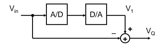
$$V_Q = V_1 - V_{in}$$
